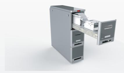
U-TP 9000C is a high-speed and space-efficient printer for boarding pass and bag tag, comprising a boarding pass printer (BPP) and baggage tag printer (BTP) in one device.
